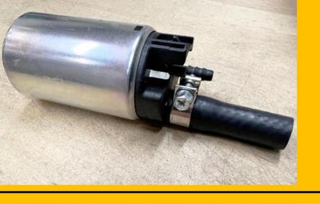
A close-up view of the Deatschwerks DW440 fuel pump. It is a cylindrical metal pump with a black rubber hose attached to the side. An EFI clamp is visible on the hose.                                                  |
