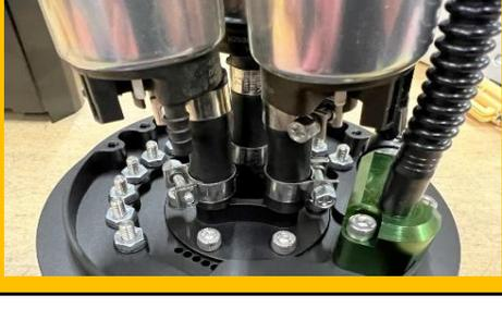
A close-up view of the fuel pump assembly installed on the collector. The pump is secured to the collector with screws, and the hose is secured to the pump with an EFI clamp. A green venturi jet pump is also visible. |
