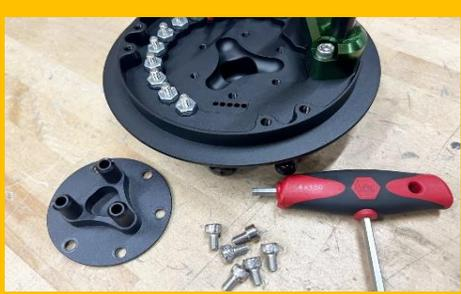
A black metal fuel pump hanger is shown being disassembled. A red-handled screwdriver is used to remove six screws from the top plate. The top plate and several screws are laid out on a wooden surface.                  |
