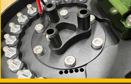
A close-up view of the fuel pump hanger showing the ports and the screws. A red-handled screwdriver is visible, and a green venturi jet pump is partially visible in the background.                                      |
