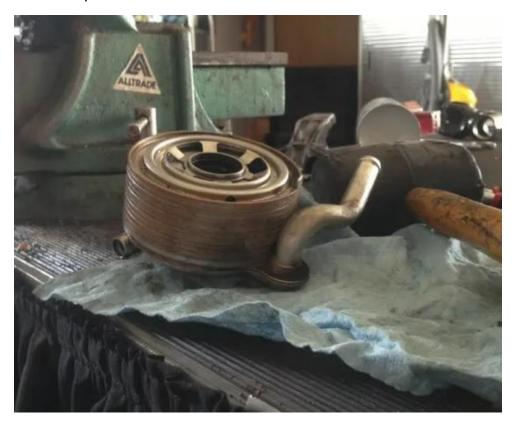
You can then reattach the oil cooler to the block using the same bolt that was used to attach the oil cooler to the mounting plate originally. Now you can reattach the coolant hoses (these may need to be trimmed):
