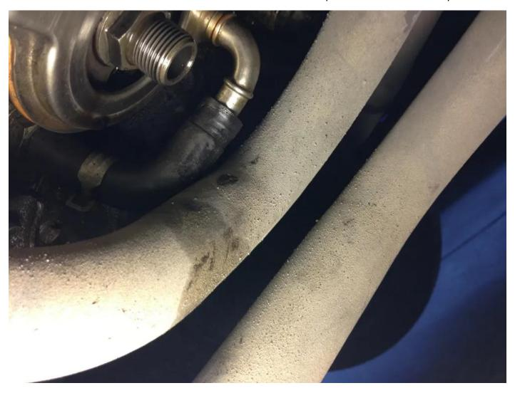
It may be necessary to modify the pipes further to allow adequate clearance between the headers. If not possible you may need to provide additional heat protection in the form of header wrap, pipe heat shield etc. to ensure the coolant hoses aren't affected by the exhaust heat.
