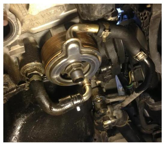
You can now proceed with installation of the headers but it is important to check clearance between the headers and coolant hoses to the oil cooler. Here is an example of how close these may be:
