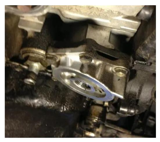
Remove the 6 bolts holding this plate to the engine and remove the plate. You will now have this bracket attached to the engine:
