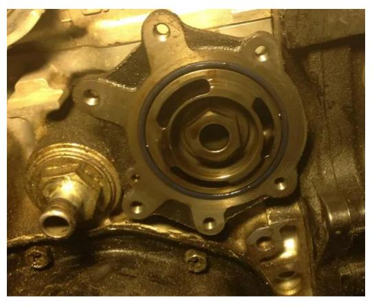
This bracket will also need to be removed so take out the large centre bolt which holds it to the engine and you can then remove the bracket.
