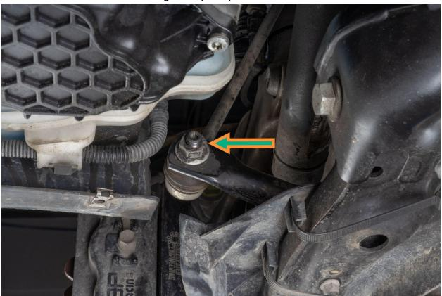
Gently pull down on the sway bar and pull link away from sway bar
