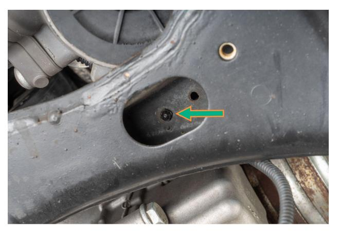
Remove 2 ride height sensor 10mm mount bolts (one on each side), then unplug the sensor. The sensor itself can hang from the subframe mount.
