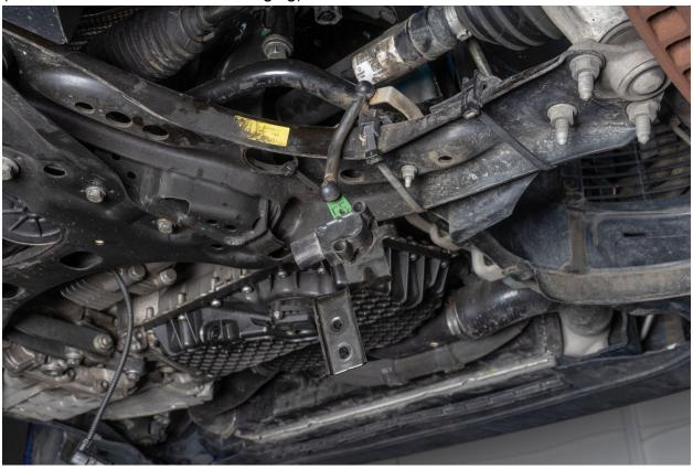
**Before** the next step, make sure you have a support system like a transmission jack to support the subframe. Remove 2 13mm downpipe mount bolts, 4 13mm bolts for the sway bar, 4 16mm and 2 18mm subframe support brackets, 4 18mm subframe bolts two of which are located on inside a hole of the subframe on the upper portion of the subframe, 2 16mm dog bone mount bolts. They are all marked below.
