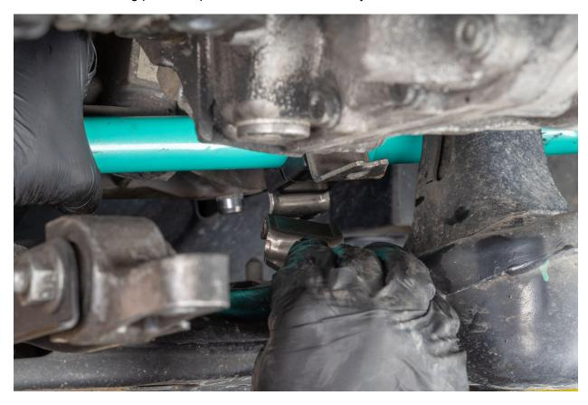
Align top and bottom mount plates with the two sway bar mount bolts that pass through the subframe, then hand tighten nuts onto bolts.
