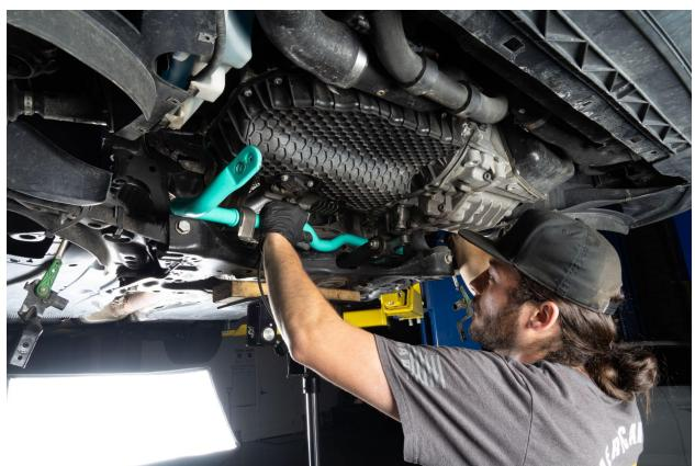
Insert lower mounting plate into position underneath IE sway bar.
