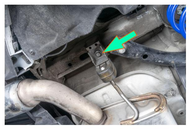
Remove OEM sway bar by dropping it out passenger side
