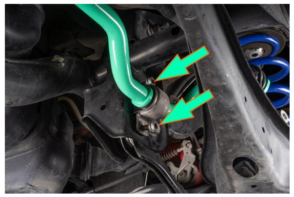
Position sway links into place and insert lower control arm bolt and nut
