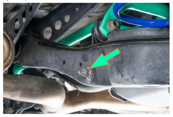
Tighten sway bar bracket bolts
