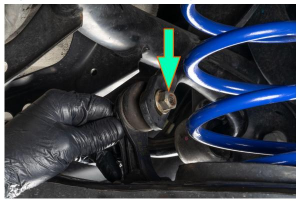
Using a 13mm wrench and socket, remove the lower sway bar link bolt and nut.
