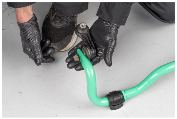
Remove OEM brackets off sway bar bushings on stock sway bar, then install on IE sway bar bushings
