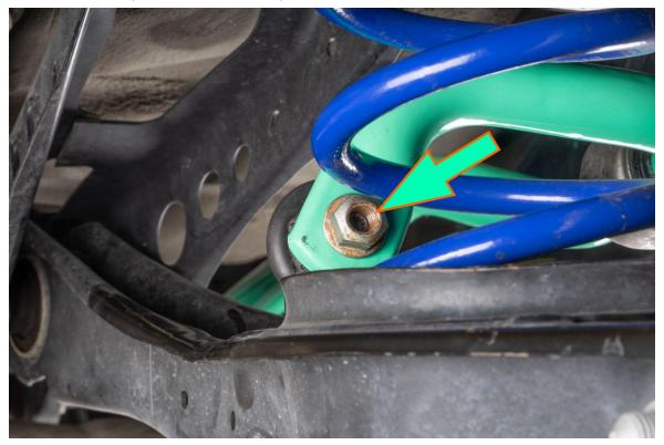
Tighten sway bar end link bolts
