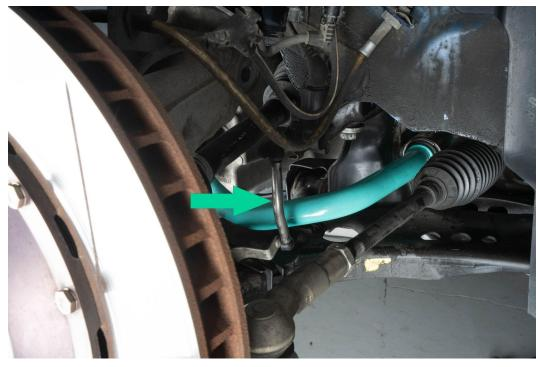
Unplug electrical connector on shock body
