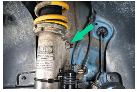
Disconnect 18mm nut connecting sway bar and shock body
