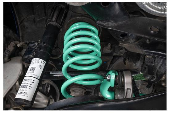
Jack up lower control arm and Reinstall two 18mm bolt connecting shock and wheel hub to lower control arm
