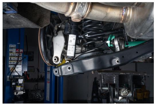
Remove spring from lower control arm and Remove upper spring cushion
