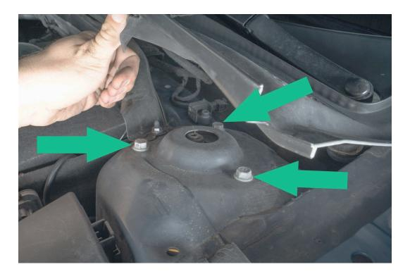
Use Jack to raise the knuckle back into the strut and reconnect the sway bar end link. Reconnect ride height level sensor.
