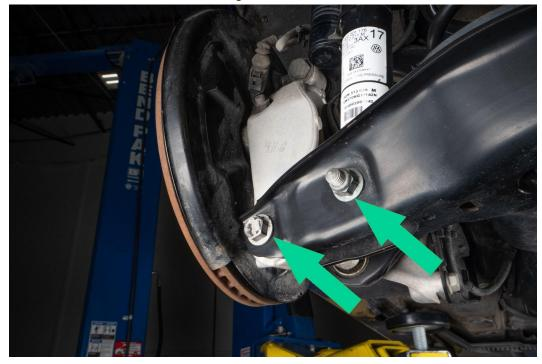
Remove two 18mm bolts connecting wheel hub and shock to lower control arm
