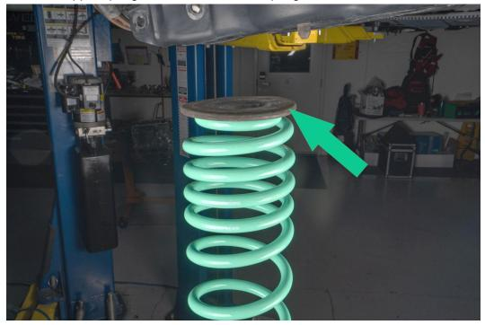
Set spring into place in lower control arm, and align top of the spring with the body
