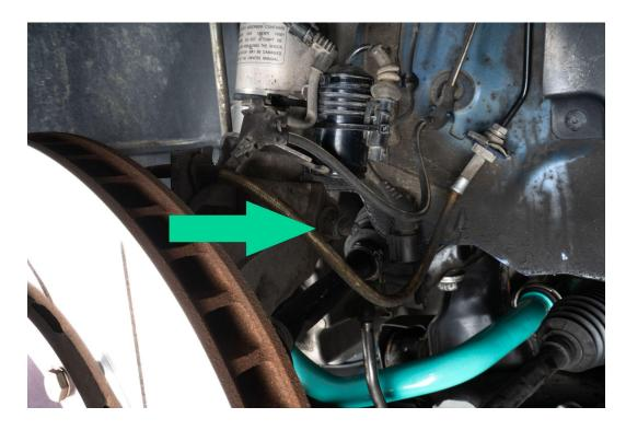
Use strut spreader to separate strut from steering knuckle
