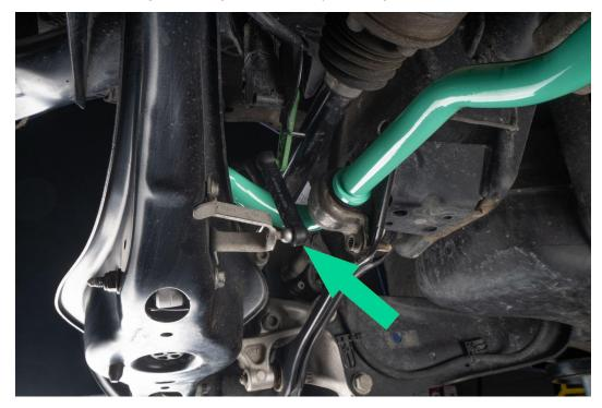
Reconnect ride height leveling sensor link by pushing onto ball
