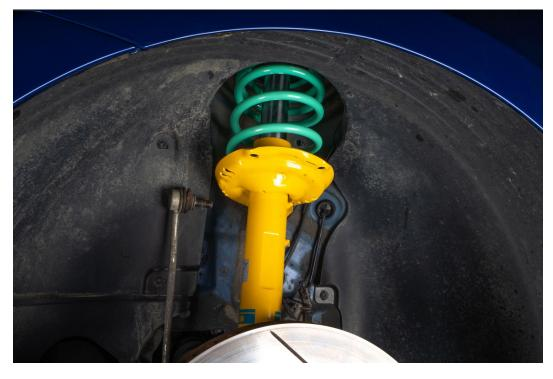
Lift strut back into place and secure upper mount bolts using a 13mm socket
