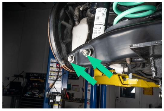
Reinstall 13MM nut and bolt securing end link to lower control arm using a 13MM socket and Wrench
