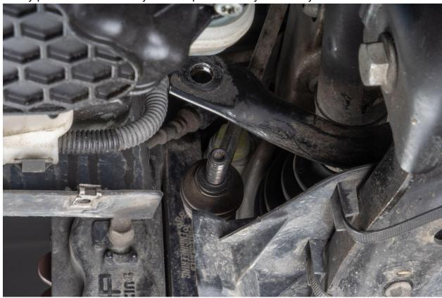
Remove oil level sensor plug from the sensor by pinching the clip, then pulling straight away from the sensor.
