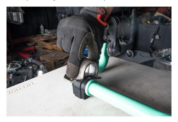
Reinstall old links on new IE sway bar using a 16MM wrench and M6 triple square. (New IE end link install instructions can be found at the end of this guide)
