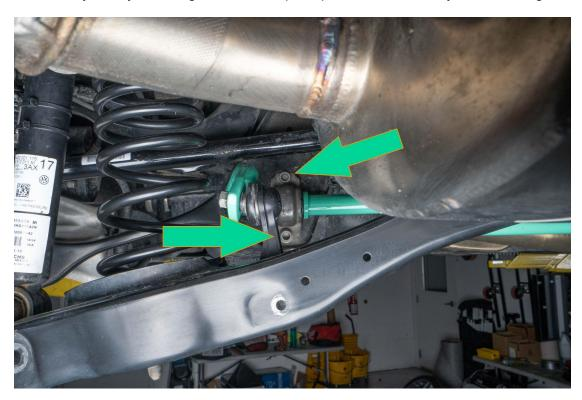
Install 2 sway bar end link 13MM bolts on lower control arms to secure end links to control arm.
