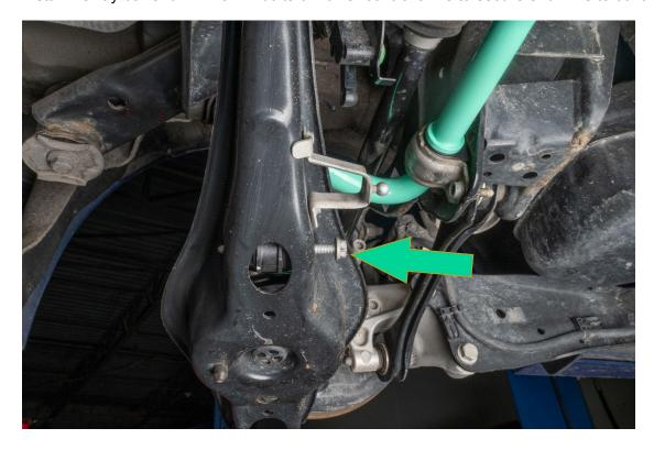
When reinstalling the lower control arm, make sure suspension parts are aligned with the body.
