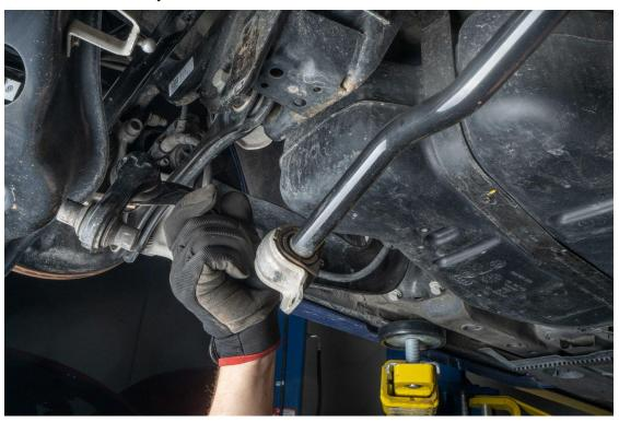
Remove the mounting bracket from the sway bar by pushing it off the bushing.
