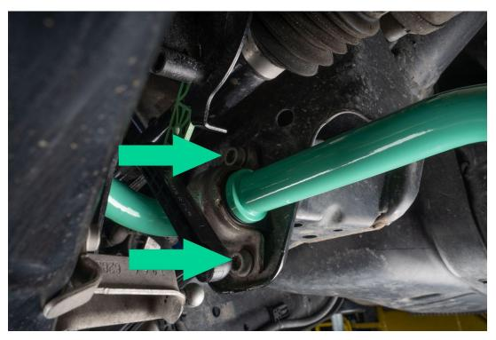
Install 13mm nut onto bolt connecting the end link and lower control arm
