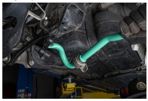
Install sway bar by screwing in 2 10MM triple square bolts into sway bar mounting bracket
