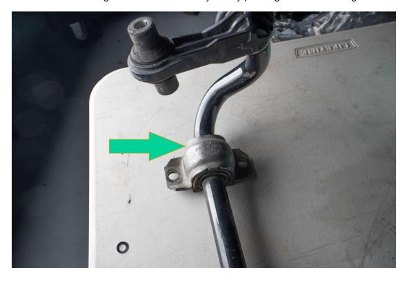
Install new sway bar bushings onto new IE sway bar.
