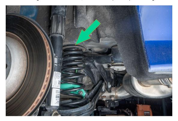
Jack up lower control arm and Install 18MM shock bolt and 18MM bolt connecting lower control arm and wheel hub.
