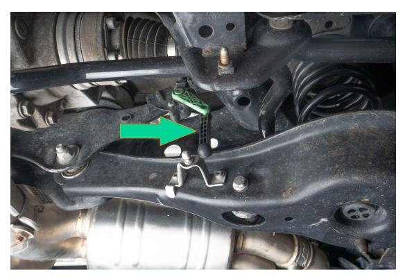
Take sway bar link bolts off using a 13MM socket and a 13MM wrench.
