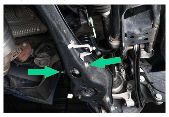
Remove sway bar mounting bracket bolts using a 10MM triple square.
