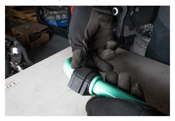
Install sway bar mounting bracket onto new IE sway bar.
