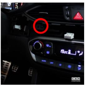
Now you can remove the two Phillips screws that hold the vent (red) and pull the vent out to the rear. Again, pay attention to the two plugs behind the hazard light switch.
