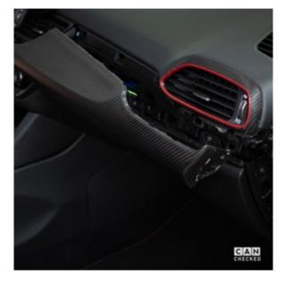
Remove the Phillips screw (red) and use the installation tool to carefully pry out the full width of the dashboard trim, around the vent nozzle to the steering column.
