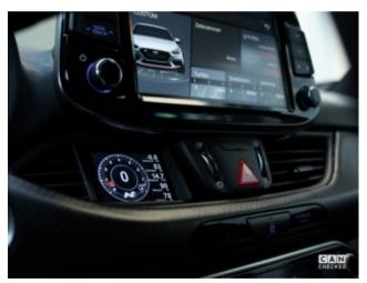
Now switch on the ignition so that the display starts. At the first start select the i30 N TRX file and confirm with "Load".
