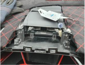
Now dismantle the fairing under the steering wheel by pulling it towards you. Don't forget to unplug the plugs on the left side and the plug and hose on the right. Then you canpull the hood side panel away to the left.
