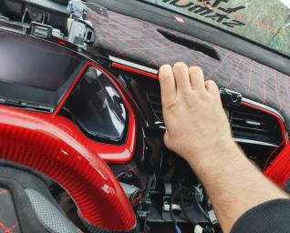
Pull out the cover so that you can release the rear plug for the hazard warning light switch. If you have solved this, you can remove the aperture completely.
