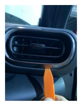
You can pull the whole vent from its place and put in on a table for further disassembling.
