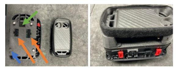
Remove the black screw from the back of the housing (blue arrow). Click in the air duct adapter and fix it with the black screw.
