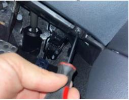
Fold the cover down and find the OBD port as well as the hole right next to it. This is where we route the cable through.
