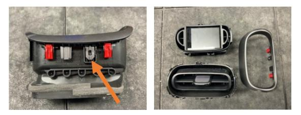
The cover fits the CANchecked unit exactly the same way. Slide the cover over the display unit and make the tabs click into their place.
