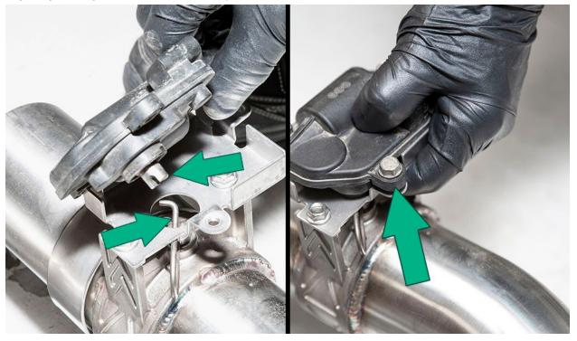
Inspect the valve actuator is properly aligned and the actuator spring is seated. Tighten bolts with 10mm socket and repeat process on opposite side valve assembly.
