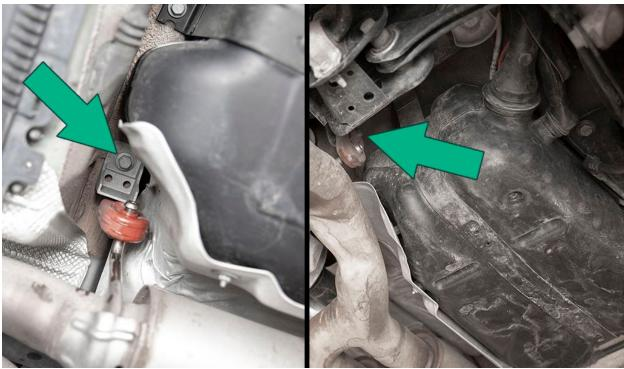
Support the catback system safely and remove both rear exhaust hangers with a 13mm socket.
