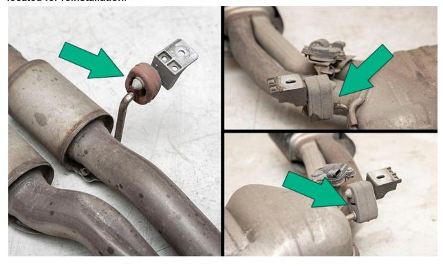
Install the rear and center exhaust hangers onto your new IE center pipe as shown.
