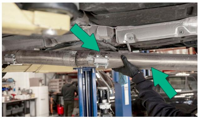
Hold the center pipe into place and reinstall the forward exhaust hanger bracket with a 13mm socket
