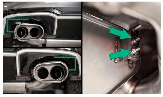
Slide the catback assembly side to side on the exhaust hangers to center the tips in the bumper. (Early Exhaust Tip design pictured below. Yours will look different, but the install is the same)
