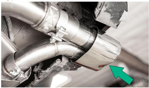
When you are happy with your tip depth on both sides and install is even, tighten all 4 band clamps firmly. *Note: make sure you are happy with install depth of tips before tightening clamps, once tightened adjustments become more difficult.*
