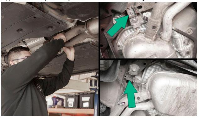
The factory exhaust is now able to be lowered out of the vehicle. An extra set of hands is recommended for safe removal. **Catback is heavy, take care removing.**
