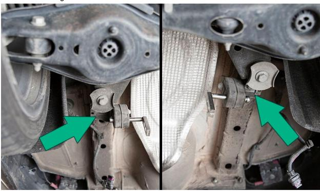
Lift the IE catback into place in the rear of the vehicle, hanging the mount studs loosely into the hanger arms.
