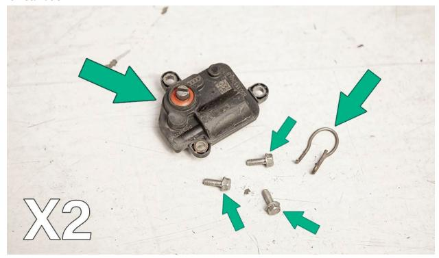
Align the spring with the actuator on the IE catback as shown below.
