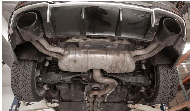
Remove the 4 nuts from the exhaust cross brace using a 13mm socket. Remove the cross brace. *Note: Your new IE catback exhaust is too large for reinstallation of this bracket.*
