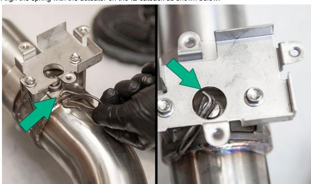
Align the valve actuator with the spring and actuator bracket. Pinch tension on the motor while finger tightening the bolts to the factory bracket.
