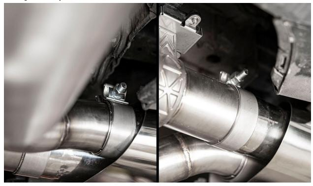
Tilt catback up and down to center the tips to personal taste, once satisfied firmly tighten the flange nuts with a 13mm socket. (Early Exhaust Tip design pictured below. Yours will look different, but the install is the same)
