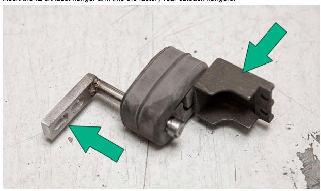
Reinstall both hanger brackets back to the chassis with a 13mm socket.
