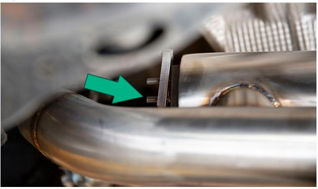
Finger tighten the four included flange nuts to both sides of the catback hanger assemblies.
