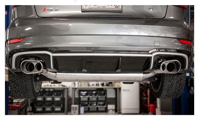
Adjust the exhaust assembly until everything sits optimally without any binding or touching and with the most ground clearance. Firmly tighten all exhaust clamps. We recommend using a strong impact gun, the clamps must stretch, but not crush the pipe to fully tighten against leaks.
