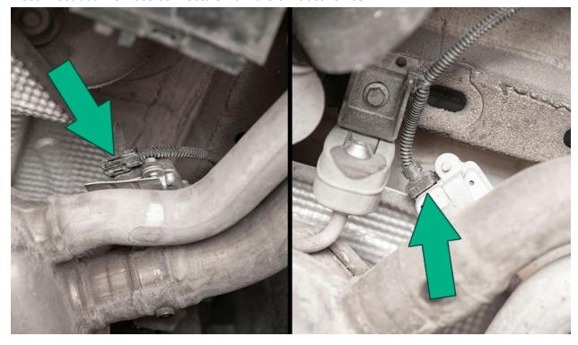
Remove the forward exhaust hanger bracket with a 13mm socket. Pry the center exhaust hanger off.
