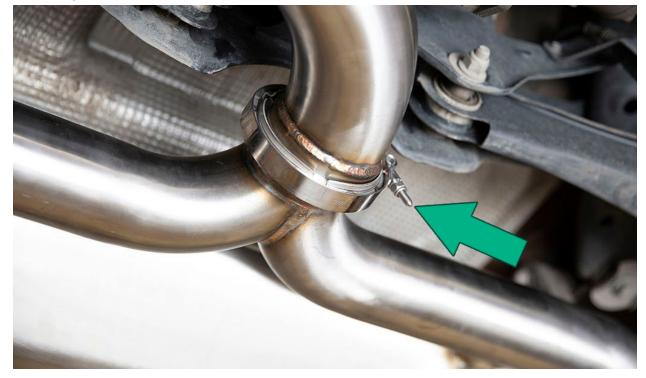
Loosely install all 4 exhaust tip band clamps onto the tail pipes.
