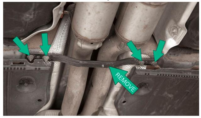
Loosen both downpipe to catback exhaust clamps with a 13mm wrench. Slide clamps onto catback to disconnect both halves.
