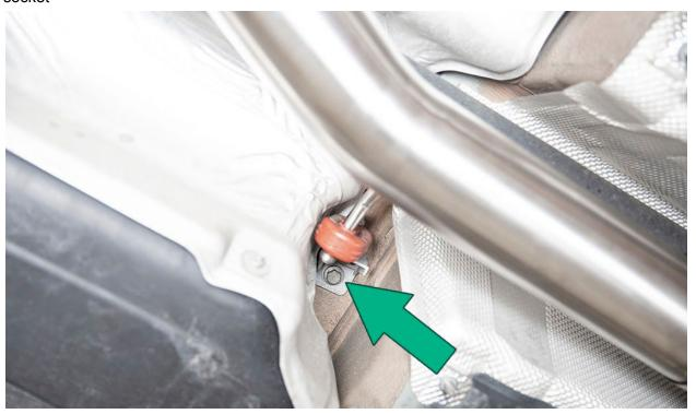
Slide the center exhaust hanger back onto the arm to secure the center pipe into place.
