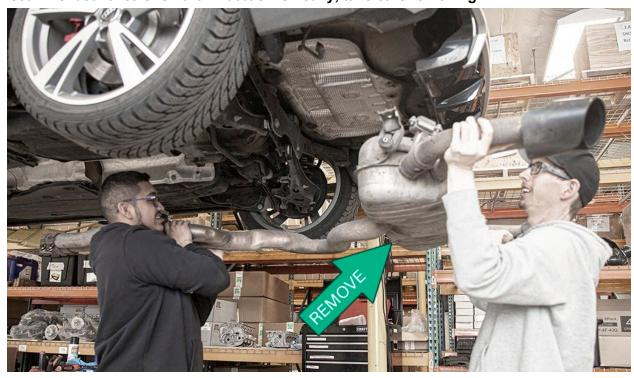
Pry all the factory exhaust hangers off the factory catback. **Keep note of where these are located for reinstallation**.
