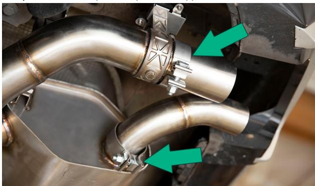
Line up the tip with the correct side of the downpipe and slide on to desired depth. There is a fair amount of adjustability, final tip depth is up to personal taste. (Early Exhaust Tip design pictured below. Yours will look different, but the install is the same)
