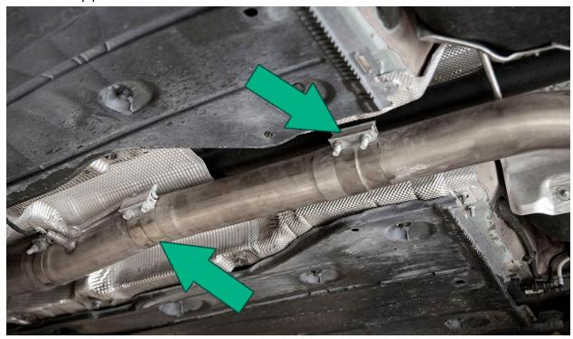
Start your car, allow it to reach temp. Listen for any exhaust leaks or signs of vibration/rubbing.
