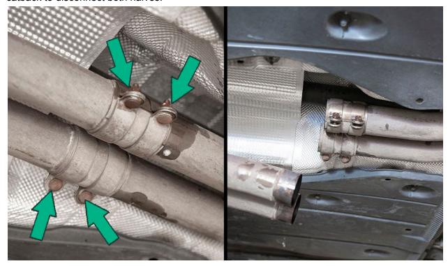
Disconnect both harness connectors from the exhaust valves..
