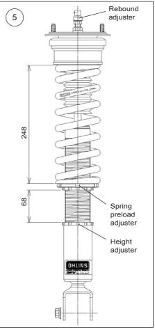
position. Moving the height adjuster outside the recommended position may cause the wheel to hit the fender liner/inner wheel well.
