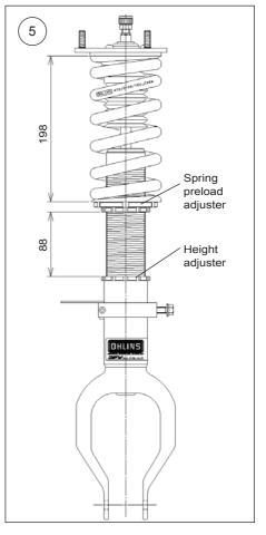
position. Moving the height adjuster outside the recommended position may cause the wheel to hit the fender liner/inner wheel well.
