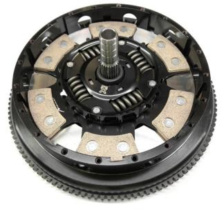
7. Install the intermediate plate, followed by the second clutch disc.
