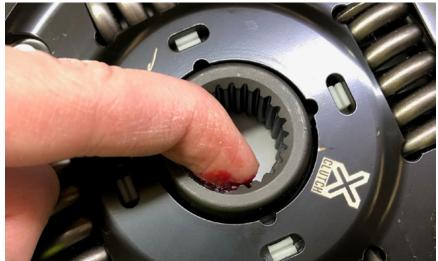
6. Install the bottom clutch disc on the flywheel with the hub/spring cage facing up. The alignment tool can be used at this point to hold the clutch disc in place, keeping it aligned with the pilot bearing.
