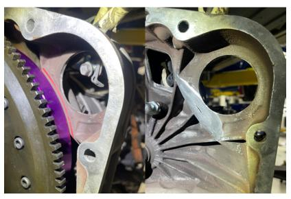
With the starter pocket modified, the clutch can be slid into the bellhousing to check for clearance. Once the clutch is mounted on the engine, mount the transmission with a few bolts and rotate the crankshaft to ensure that the clutch does not interfere with the bellhousing.
