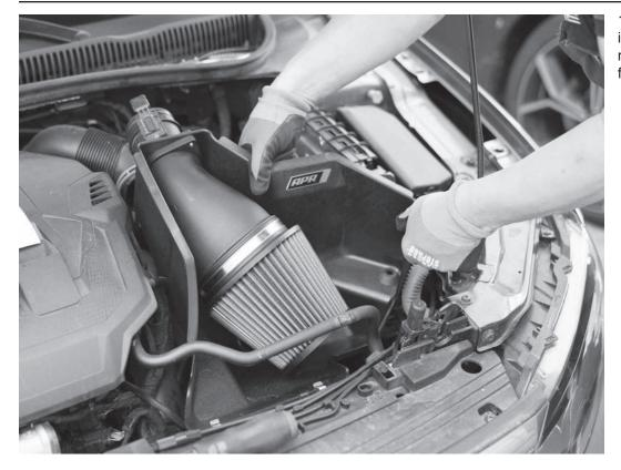
17) Place the APR airbox assembly into the car, making sure the three rubber mounts connect with the three factory mounting posts on the car.
