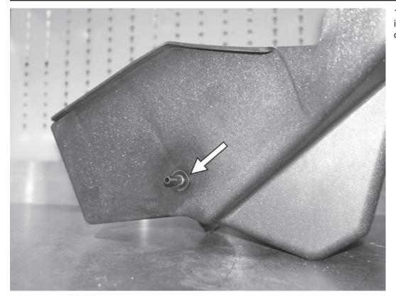
11) Install the straight barbed fitting into the rubber grommet on the side of the APR heat shield. Use
