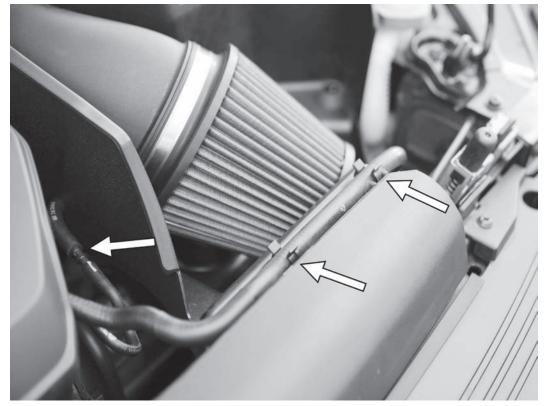
21) Reattach the coolant hose into the two clips on top of the factory airbox inlet. Connect the factory vacuum line that went to the side of the factory airbox onto the straight barb fitting on the side of the APR airbox.
