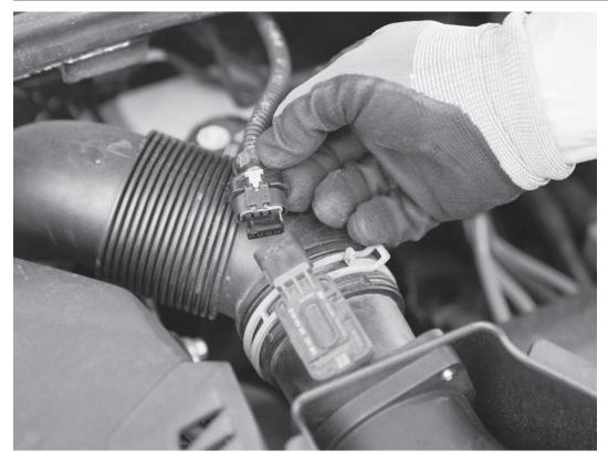
19) If equipped, reconnect the electrical connector to the MAF sensor. Be sure to slide the white tab on the connector forward to lock the connector in place.
