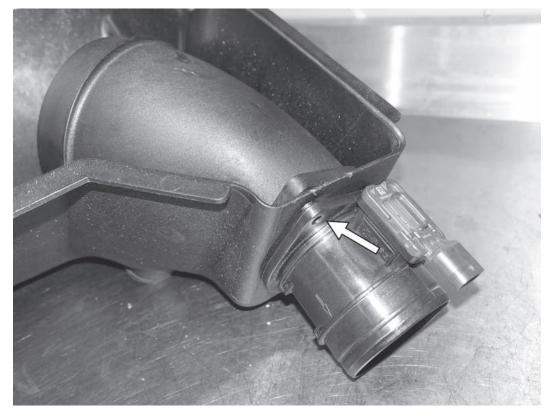
15) Place the MAF sensor or the APR MAF adapter into the back of the APR heat shield. Orient and install the APR filter adapter onto the MAF sensor from the other side of the heat shield.
