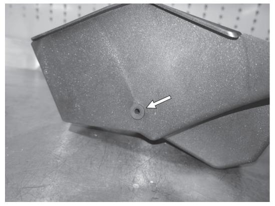
9) Using an evaporating lubricant, install the bigger of the two smaller rubber grommets into the side of the APR heat shield.
